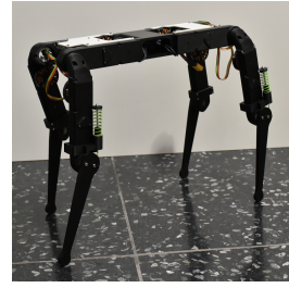
Fig. 3. Spring loaded knee joint with a bidirectional actuator, quadrupedal platform, robot modified from the Open Dynamic Robot Initiative [1].
